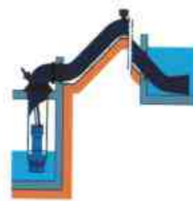
Installation of wellbore bend pipe
